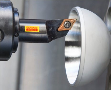
Holder: A20M-ADXCL 11-R Insert: DCGT 11T308-UM 1115
