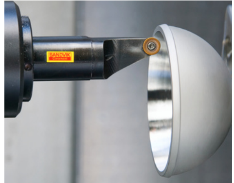
Holder: A20M-SRXDL 08-R Insert: R300-0828E-PL 1030
